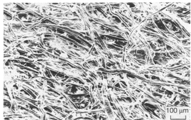
Figure 9 Scanning electron micrograph of the ashless filter paper used to stack and press film before pyrolysis.
